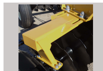
"W" Series with heavy 4" x 6" tubing and bearing hangers
