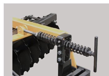
Self-leveling spring cushioned with hand crank
